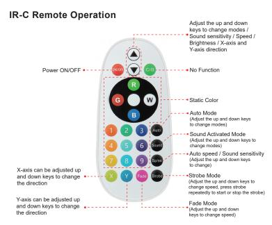
Note: 1-9 static colors can not be adjusted by up and down keys to adjust the brightness
