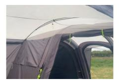
Once connected to the vehicle and the awning is fully pegged out, assemble pole and fit in via the Velcro fittings attached to awning
