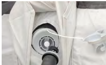
*Fig 1. - Valve position is changed with the white push button at the centre, there are two positions. Closed/Inflate - button will be taller/proud of housing | Open/Deflate - button will be depressed/shorter Pump Hose is a bayonet style connection and locks in place with a twist
