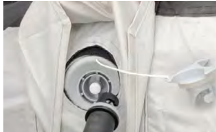
*Fig 1. - Valve position is changed with the white push button at the centre, there are two positions. Closed/Inflate - button will be taller/prod of housing | Open/Deflate - button will be depressed/shorter Pump Hose is a bayonet style connection and locks in place with a twist
