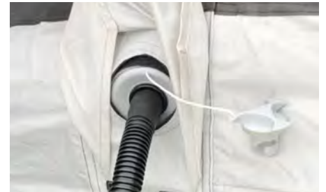
*Fig 1. - Valve position is changed with the white push button at the centre, there are two positions. Closed/Inflate - button will be taller/proud of housing | Open/Deflate - button will be depressed/shorter Pump Hose is a bayonet style connection and locks in place with a twist
