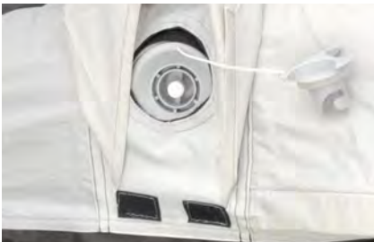
*Fig 1. - Valve position is changed with the white push button at the centre, there are two positions. Closed/Inflate - button will be taller/proud of housing | Open/Deflate - button will be depressed/shorter Pump Hose is a bayonet style connection and locks in place with a twist
