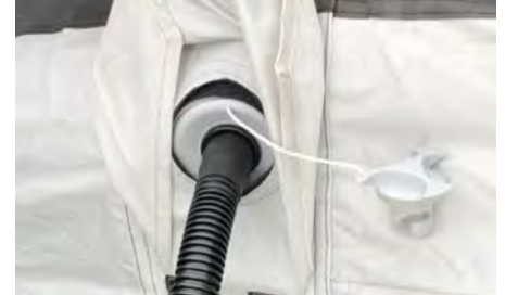
*Fig 1. - Valve position is changed with the white push button at the centre, there are two positions. Closed/Inflate - button will be taller/protrude of housing | Open/Deflate - button will be depressed/shorter Pump Hose is a bayonet style connection and locks in place with a twist
