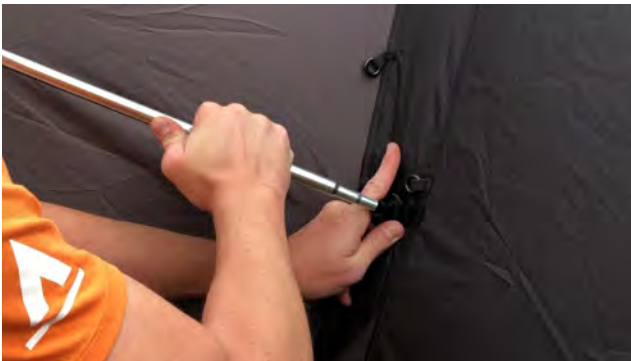
15. Locate end of pole into plastic cup
