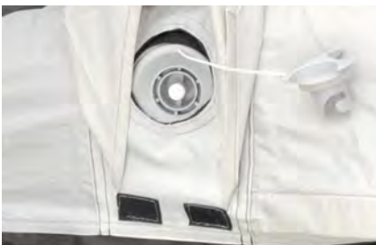
*Fig 1. - Valve position is changed with the white push button at the centre, there are two positions. Closed/Inflate - button will be taller/protruding of housing | Open/Deflate - button will be depressed/shorter Pump Hose is a bayonet style connection and locks in place with a twist
