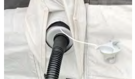
*Fig 1. - Valve position is changed with the white push button at the centre, there are two positions. Closed/Inflate - button will be taller/protruding of housing | Open/Deflate - button will be depressed/shorter Pump Hose is a bayonet style connection and locks in place with a twist
