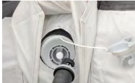
*Fig 1. - Valve position is changed with the white push button at the centre, there are two positions. Closed/Inflate - button will be taller/protruding of housing | Open/Deflate - button will be depressed/shorter Pump Hose is a bayonet style connection and locks in place with a twist
