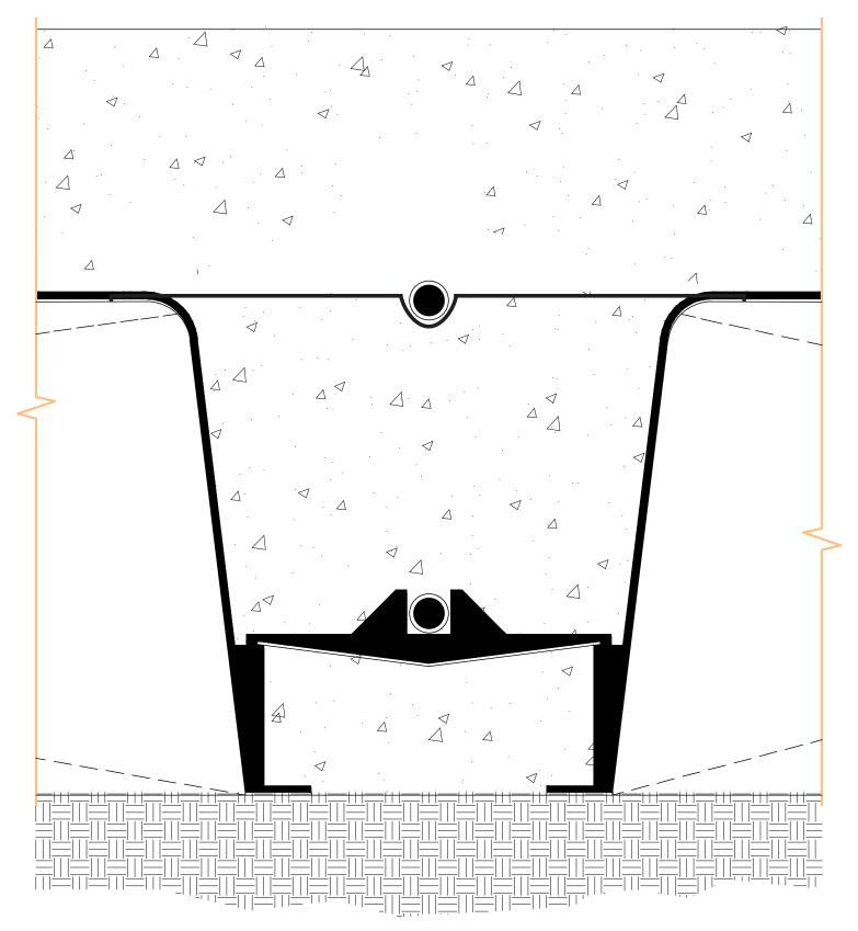
\*Profile view of Post Tension Cables perfectly aligned using a Wafflebox Tendon Clip.
