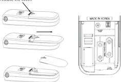
Note: Make sure to insert the batteries in the proper position of positive(+) and negative(-) as indicated.
