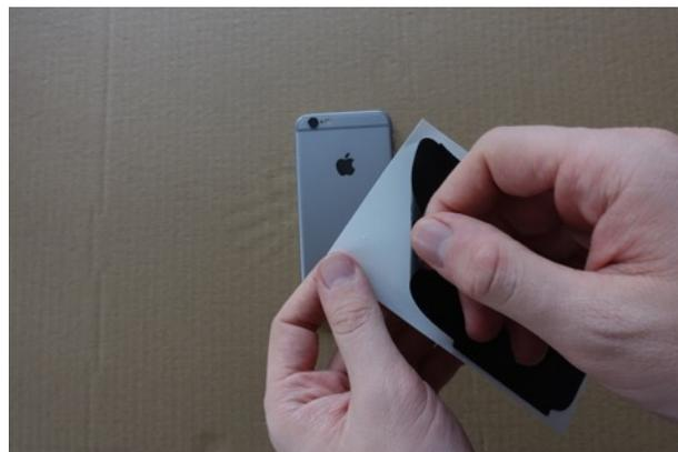
The skin should be laid down on the iPhone gradually from the top to the bottom of the phone. Start by fitting up the holes for the camera/flash, then the Apple logo, and the bottom at last.
