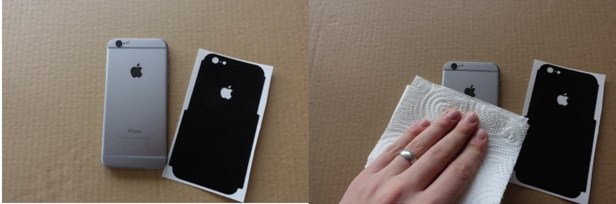
2. Separate the skin from the back-paper and place it on the iPhone. The process consists of two steps. First the backside is placed, then the sides are done with a hair dryer.
