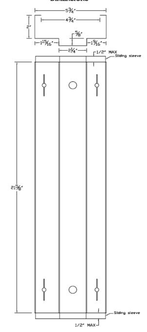
NOTE: THE EXISTING JAMB DIMENSION SHOULD BE CHECKED AGAINST THIS SPECIFICATION PRIOR TO USING THE JAMB PATCH PRODUCT.
