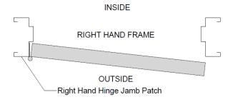
NOTE: THE EXISTING FRAME HANDING SHOULD BE CHECKED AGAINST THIS GUIDE PRIOR TO USING THE JAMB PATCH PRODUCT.
