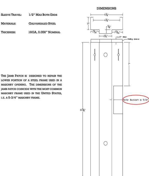
NOTE: THE EXISTING JAMB DIMENSION SHOULD BE CHECKED AGAINST THIS SPECIFICATION PRIOR TO USING THE JAMB PATCH PRODUCT.
