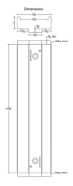
NOTE: THE EXISTING JAMB DIMENSION SHOULD BE CHECKED AGAINST THIS SPECIFICATION PRIOR TO USING THE JAMB PATCH PRODUCT.
