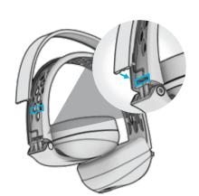
REMOVING: Fold in the hinges and locate the Tension Band groove. Pull outward with your finger to unlock.
