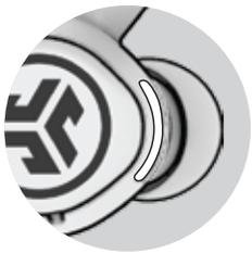
After earbuds are powered on and connected, **white pulsing lights** will turn off after 30 seconds. They will turn back on when pressing any button function.
