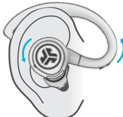
**2** Locate the earbud to the ear canal and rotate inward.
