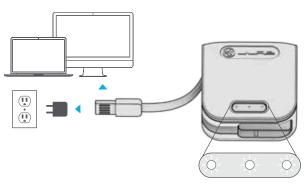
LEDs **pulse white** when charging and **turn solid white** when fully charged.
