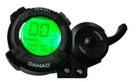
Press 🕑 Power button to Turn on or Turn off Display; 💷 Show battery
