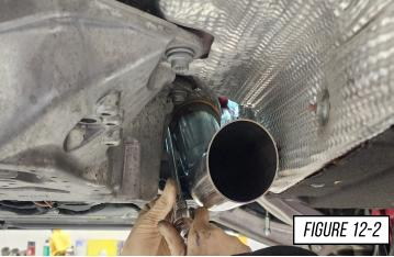
Install your AWE mid section (**E90**) with the flat side of the can facing down, as shown below in **Figure 13-1**. Bottom out the two slip fits of the mid section onto the downpipe legs (**E88**), and (**E89**). Snug the clamps, but do not fully tighten at this time.
