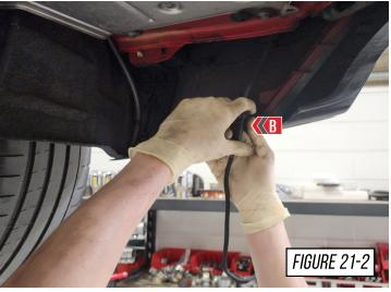
Install your AWE driver side switchpath section (**E94**), by first sliding a provided clamp over the expanded joint.
