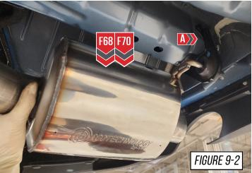
To install the exhaust tips with integrated clamps, first, attach the exhaust tip in the proper orientation onto the exhaust outlet tube.
