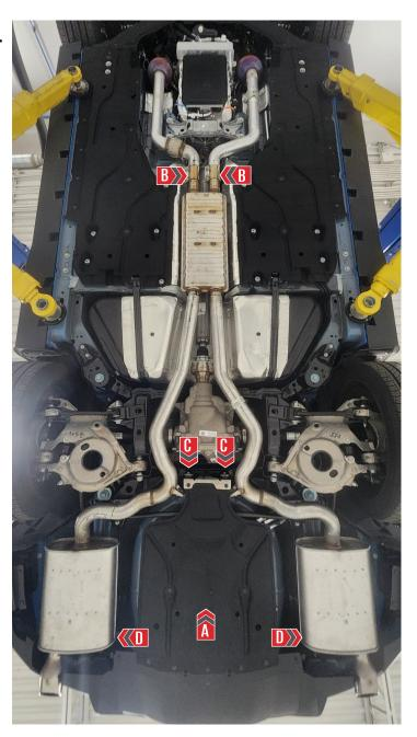
Gather your AWE H-Pipe (**F66**), and your AWE H-Pipe OEM adapters (**F65**). Slide the OEM adapters into the expanded ends, as shown in **Figure 2**.
