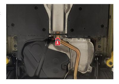
With the complete AWE exhaust system installed, all clamps tightened and the tips aligned. It is now recommended to drive the car to allow the exhaust to heat cycle.
