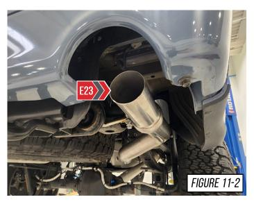
To install the exhaust tips with integrated clamps, first, attach the exhaust tip in the proper orientation onto the exhaust outlet tube.
