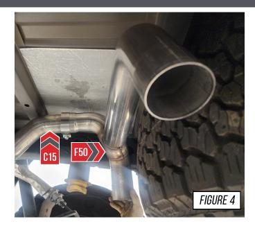
It is crucial to install each section and Accu-Seal clamp correctly to prevent loose joints, exhaust leaks between the tubing connections, and rattles.
