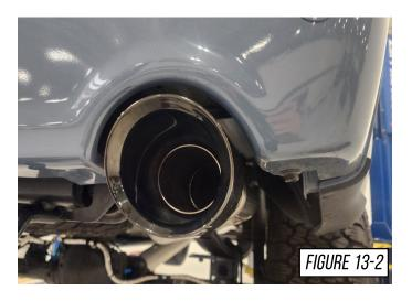
Make your final adjustments to the tips to ensure they are in a position you like. Once the desired positioning is achieved work from the front of the car to the back, tightening all the clamps fully and ensuring there is proper clearance of the chassis and braces.
