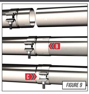
Install the AWE Mid Section (part **C15**) by securing the hanger bars into their respective brackets, then slip one of the supplied 3.0" Band clamps over the inlet end and connect it to the outlet of the preceding tube. **Figure 10.**
