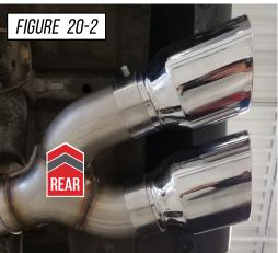
For **dual side** tip outlets, use the supplied 3-inch Band Clamps (TAS300) to install the 5" straight cut tips to the same specifications outlined in **Step 9**.
