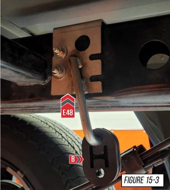
Install the rear axle tubes, Drivers side (**part C19**) and passenger side (**part C20**). Use the supplied 3.0" Band Clamps (**A**) and rubber exhaust isolators (**B**) shown in Figure 15.
