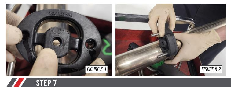
With the OE hanger installed on your AWE resonated mid pipe (**F28**), gather a provided clamp and slide it over the expanded end of the tube.
