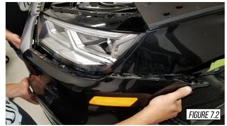
Finish detaching the tabs holding the bumper cover in place by pulling straight out, away from the vehicle.
