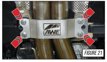
Install the remaining chassis braces starting with the driver side since the passenger side must overlap it.
