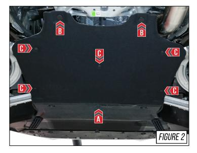
Next, remove the central underbody panels in order to gain access to the chassis brace bolts toward the front of the vehicle.
