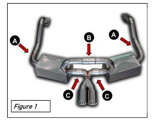
On 2009-12 Cayman/Boxster ONLY: install the enclosed aluminum 3/8" spacers between the DRIVER SIDE factory hanger bracket and the corresponding bracket on the AWE Tuning muffler. Substitute the factory bolts with enclosed M8 bolts and washers
