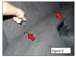
Carefully pry off the passenger side speaker cover as shown.
