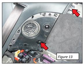
Remove the lower A pillar trim and pull back the carpet to expose the fuse box.
