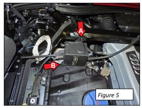
Flip the AWE Tuning SwitchPath™ Control Unit on its side, with the welded bracket facing the driver's side (coupe only).
