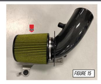
Install the AWE carbon fiber intake filter section into the vehicle, by pushing the OEM rubber mounting grommets into place and aligning the silicone flex tube, as shown in Figure 16.
