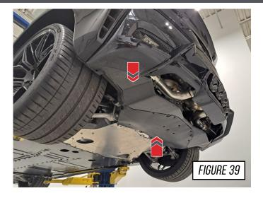
With the complete AWE exhaust system installed, all clamps tightened and the tips aligned. It is now recommended to drive the car to allow the exhaust to heat cycle.
