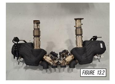
Remove the OE valve motor and arm from the OE exhaust. First remove the clip securing the ball joint (**A**), then pull ball joint off of OE valve, next remove the 3 bolts (**B**) holding the motor to the exhaust, as shown in **Figure 14.1**.
