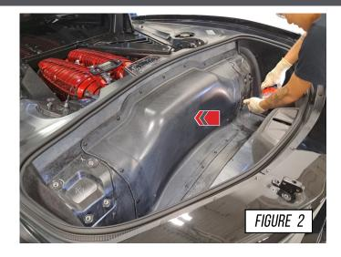
Spray both the driver and passenger side flange with penetrating oil, to aid in removal. Let the penetrating oil soak while removing the bumper.
