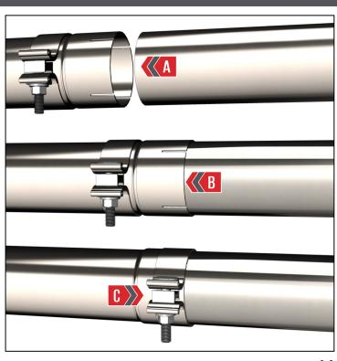
Install your AWE X pipe section (**F55**) with 2 supplied clamps and the slip fits over both AWE valve sections, as shown in **Figure 21**.
