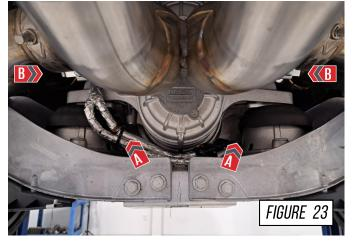
Gather the one long 14" cable tie, fold the cable tie in half and go <u>over</u> and <u>around</u> the wiring harness (**A**), there is a small hole in the chassis, slide both ends of the cable tie through that hole (**B**), secure the cable tie around the bar on the chassis (**C**), as shown in **Figure 24.1** and **24.2**.
