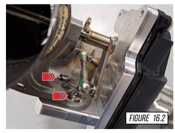
Secure the ball joint, as shown at (B) in Figure **17**.
