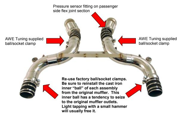
The AWE Tuning Straight Pipe System eliminates the use of the factory vacuum actuated muffler flaps. After disconnecting the vacuum lines from the factory muffler, cap them by inserting the supplied screws.
