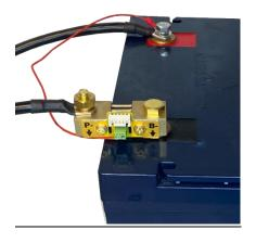
7. Ensure all connections are clean of corrosion, they are tight and secure.
