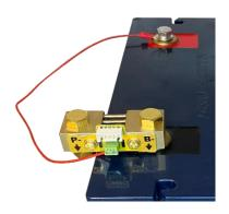
5. Connect your other parallel connections, and negative charger connection to the "P-" on the shunt. Reverse the bolt so the head side is down and the washer, lock washer and nut are on top.
