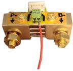
3. Install the shunt, "B-" side <u>flush</u> with the main negative terminal. Use the provided bolt with the washer and lock washer on top.
