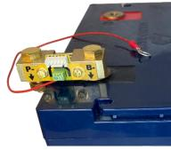
4. Attach the small positive lead eyelet to the same positive terminal on the battery.
