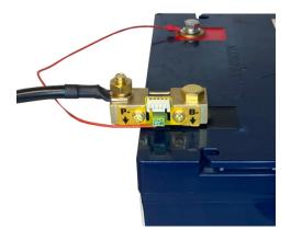
Note: It is important to install your highest, current drawing cables (larger gauge) facing the terminal directly and installing the smaller drawing cables (smaller gauge) furthest from the battery terminal.
