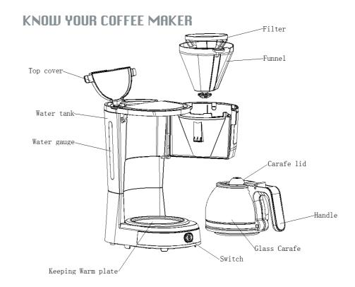
Electrical parameters: 120V~ 60Hz 700W
