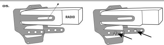
Install the radio into the mount using the allen head bolts that came with your radio.
