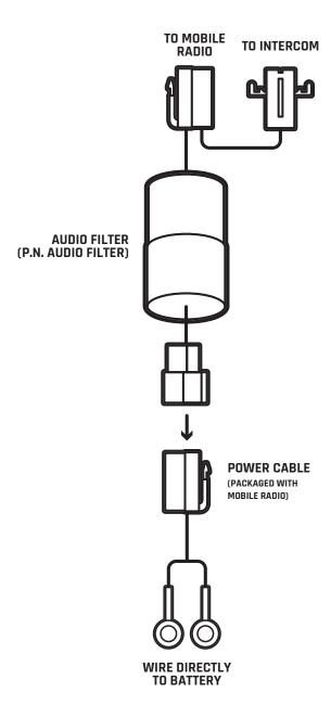
NOTE: Cables and connections are not to scale.
