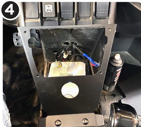
Position the top of the mount as shown in this diagram above and reinstall the 2 torx bolts. **IMPORTANT: *With the console support pillars removed, the upper dash will sag slightly. It's important to raise and realign the dash. Vice grips may be a good option to hold the dash and the mount in place.*** Once lined up as shown in the left photo above, drill holes in the left and right side using a 1/4" drill bit. Put bolts through the holes you just drilled and attach the mount to the upper dash.
