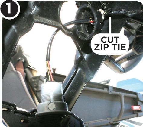
Start by reaching behind and loosen the nut that is securing the start/stop button. On the backside, there is a small zip tie securing the start/stop wires to the plastic dash that will need to be cut to release the wires. Unplug and remove the start/stop button.
