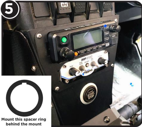
Mount the Start/Stop Button. Included in the kit is a round spacer shaped like the start/stop button. That will be added to the back of the button before the factory plastic spacer and nut.
