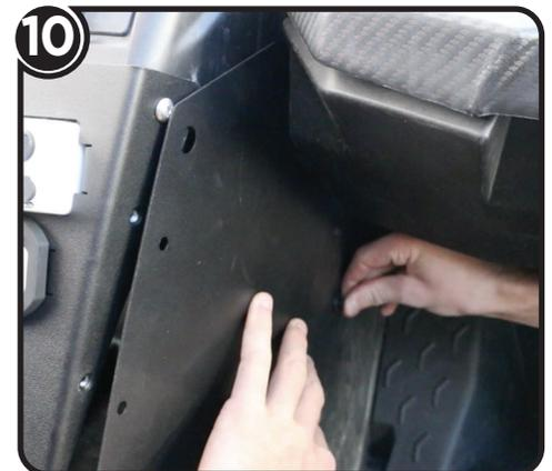
Follow the next step if you are installing the optional side panels. On the passenger side, start by removing two plastic rivets towards the back, closest to the floorboard. Next, place the side panel in place and insert the plastic rivets back into their holes. The panel can be lined up for the front bolts and secured. On the driver side, attach the 2 side bolts and secure.
