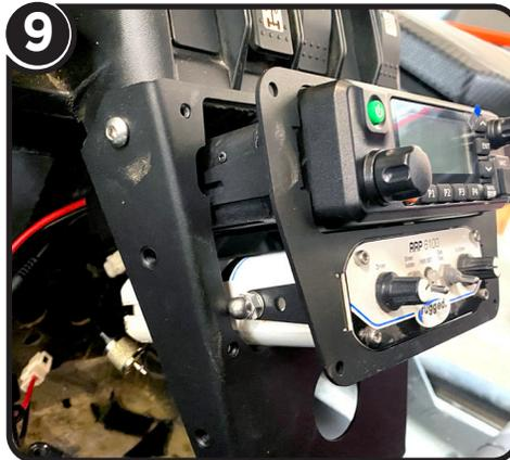
Plug all communications cables into the intercom paying close attention to the driver and co-driver ports. The pigtail with a chrome 5-Pin connector will plug into the pigtail on the back of the radio. Don't forget to hook up the antenna cable to the radio! Once all cabling is plugged in, slide the insert into the mount and install the 4 screws.
