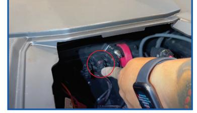
Be sure to connect the ground wire to the ground bolt on the vehiclev.
