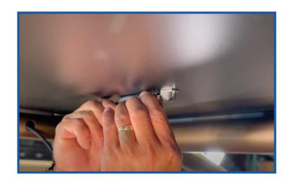
Secure the Antenna. Be sure not to over tighten.
