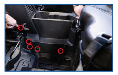
To create more working space, remove the bolts securing the front seat belts.
