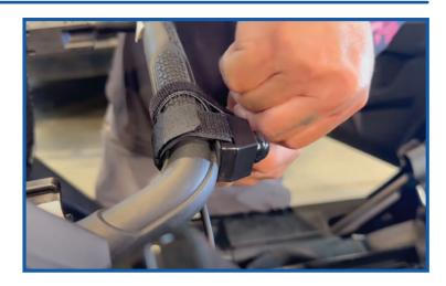
Secure the coil cord PTT to the steering wheel, adding a strain relief loop.
