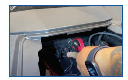
Insert the mounted Mobile radio into the dash.
