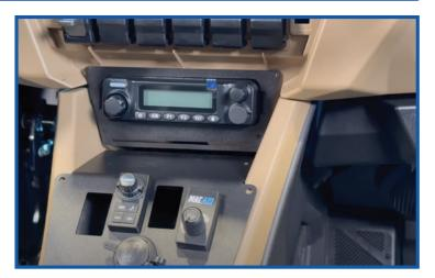
Secure the lower optional panel and route all necessary cables.
