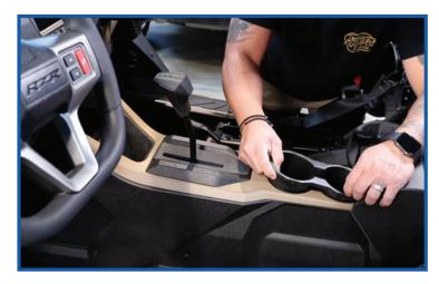
Remove the bolt beneath the rubber gasket and work the gasket loose around the gearshift.
