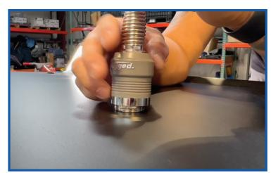
Once the antenna is installed, loosen several bolts holding the roof. This will allow us to slip R-Wraps around the roll cage and secure the COAX cable in place. Retighten all the roof bolts after cleaning cabling up with R-WRAPS.
