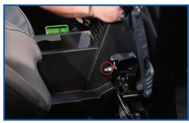
Remove bolts beneath the plastic panels under the rear seats, easing tension on the rear center console.
