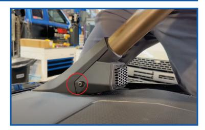
Using a wire snake, gently pull the antenna coax cable (small connector to the roof) up the roll cage, through the roll cage hole at the bottom of the A-Pillar.
