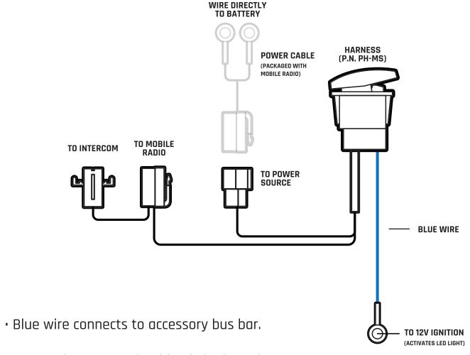
• Connection source should only be hot when ignition is turned on.
