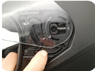
use the tab to release the shield from the helmet
