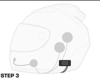
Affix the helmet kit jack box on the exterior of the helmet using the 3M adhesive. Optimal location shown above. Adjust as necessary to accommodate cable lengths.
