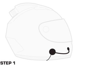
Using the 3M adhesive, affix mic boom to the interior of your helmet positioning the mic directly in front of your lips. The adhesive should mount to the shell, ON THE LEFT SIDE under the helmet liner. (LEFT REFERS TO LEFT SIDE AS IF YOU WERE WEARING THE HELMET)
