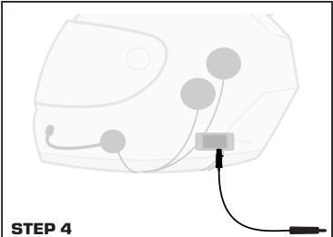
Attach the appropriate adapter cable for your intercom. The cable with the grey modled plug is for use with STEREO intercoms only. The cable with the blue molded plug is for all standard OFFROAD intercoms.
