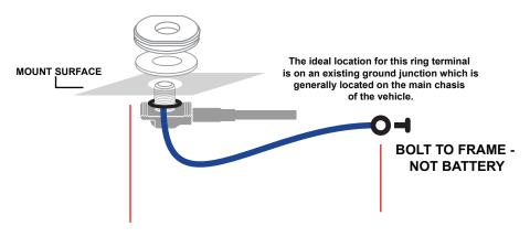
Scrape away paint/powder coating on bottom side of mount surface and ring location to provide good metal contact.
