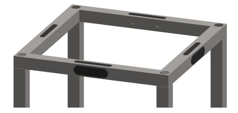
**6.** Install the **Top Plate** onto the top Frame and fully tighten the **Frame Screws** until just past snug. Do not overtighten.
