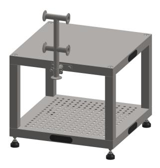
**5.** Install the four **Micro Adjust Valves** onto the **Tubing Tree** and secure with a 1.5" Tri-Clamp as shown. The bottom port of the **Tubing Tree** connects to the pump outlet tubing (sold-separately).
