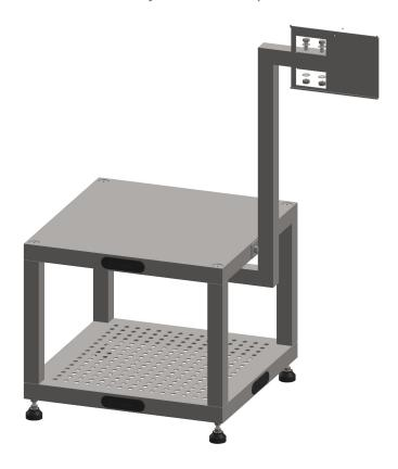
2. Fasten the **eController Mount** to the **Side Arm** using the included 3/8"-16x2-1/4" screw, nut, and washer assembly. Fully tighten the hardware until just past snug. Do not overtighten.
