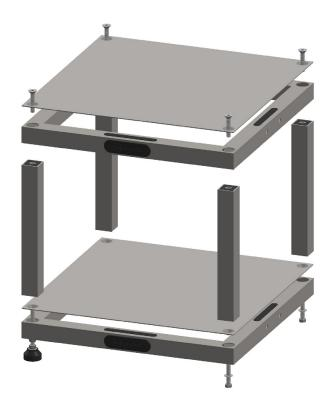
**3.** Lay both **Brew Cubes** on their side and assemble the (4) 3/8"-16x3-1/2" screw, washer, and nut assemblies on the top and bottom holes as shown. Wait to fully tighten the hardware until all four screws have been installed. Fully tighten the hardware until just past snug. Do not overtighten.
