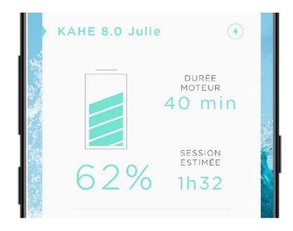
When not in use for several months, your battery should be stored with a charge level between 50% and 75%. This will prolong its life to the maximum. Because a stored battery charged at 100% sees its performance degrade more quickly.
