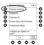
3. Adjust display and return to main screen (see Start-Up," Adjust Display Contrast" procedure).
