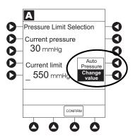
6. Verify correct pressure limit input and press **CONFIRM** soft key.
