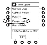
4. Press either **Pump** or **Selectable** pressure soft key. If **Selectable** is pressed, continue with next step; otherwise, proceed to last step.
