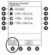
2. Pump module: To view primary and secondary volume(s) infused, press **PRI/SEC VOLUME** soft key.
