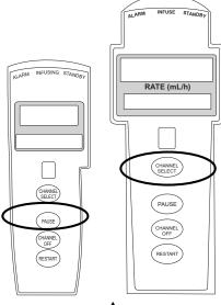
5. Syringe module: Select syringe type and size, as follows; otherwise, proceed to step  $6.^{\circ}$
