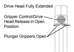
3. Insert syringe (from front of instrument) by sliding flat edge of syringe barrel flange between barrel flange grippers.
