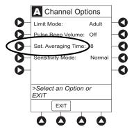
To change Saturation Averaging Time, press applicable soft key. Selectable options are 2, 4, 8, 10, 12, 14, and 16 seconds.
