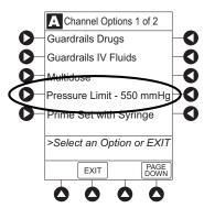
5. To enter a new pressure limit value, press **Change Value** soft key. <sup>①</sup>
