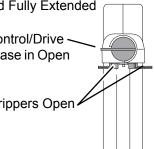
4. Insert syringe (from front of instrument) by sliding flat edge of syringe barrel flange between barrel flange grippers.
