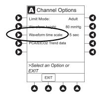
2. To change **Waveform Time Scale**, select applicable time scale.
