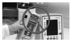
7. Fully inspect the instrument during each cleaning. Look for any visible external damage such as a cracked or broken door, handle, or latch. Open the door of each pump module and inspect the platen and hinge for cracks or other damage.
