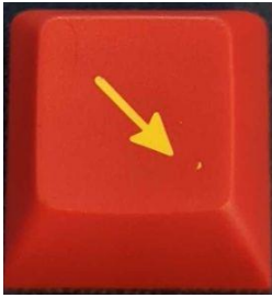
Underside plastic showing through the topside plastic
