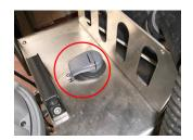
Lift the cap to the water reservoir, insert the red funnel and fill with ONLY cold clean tap water.
