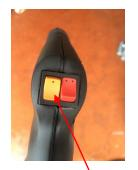
Push the orange button into the ON position and the chemical will be released periodically when the trigger is pressed on the pistol grip to release the steam
