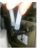
Firmly connect the chemical filler tubes from the chemical machine
