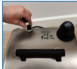
Open the steam output regulator knob and regulate it to the required amount of steam.
