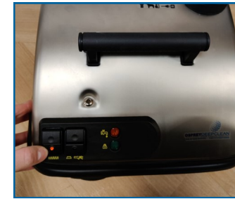
Switch on the main switch. The boiler ready lamp (green lamp) will light up when ready for use.
