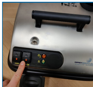
Now the machine is ready for use: Activate the steam switch.
