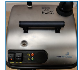
Switch on the main switch. The boiler ready lamp (green lamp) will light up when ready for use.
