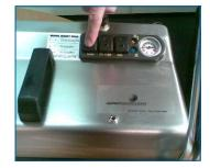
Switch on the main switch. The boiler ready lamp (green lamp) will light up And blink. When the lamp lights up continuously, the machine is ready
