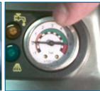
De-pressure the boiler: Press the left switch of the pistol grip and the trigger (red switch underneath the pistol grip), untill the pressure gauge shows 0 bar.
