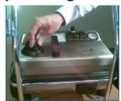
Push down on pressure safety cap then turn the cap anti-clockwise to unscrew.
