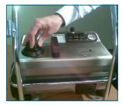
Push down on the tank cap and turn it clockwise to screw it shut firmly.
