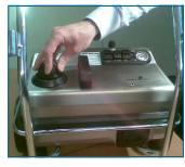
Push down on the tank cap and turn it clockwise to screw it shut firmly.
